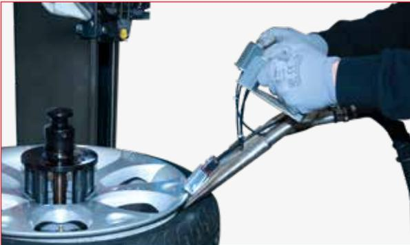
TI system Kit: version for "AUTOMATIC" and "Manual" edge clamping
